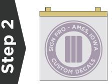
When the graphic is in the correct position, apply a long strip of masking tape to the top edge (or side) to create a "hinge".
