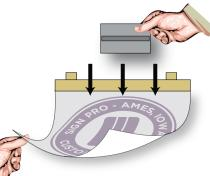
Using a vinyl squeegee or similar piece of plastic, slowly work your way across the graphic starting at the hinge while holding the bottom end of the graphic away from the surface with your free hand.
